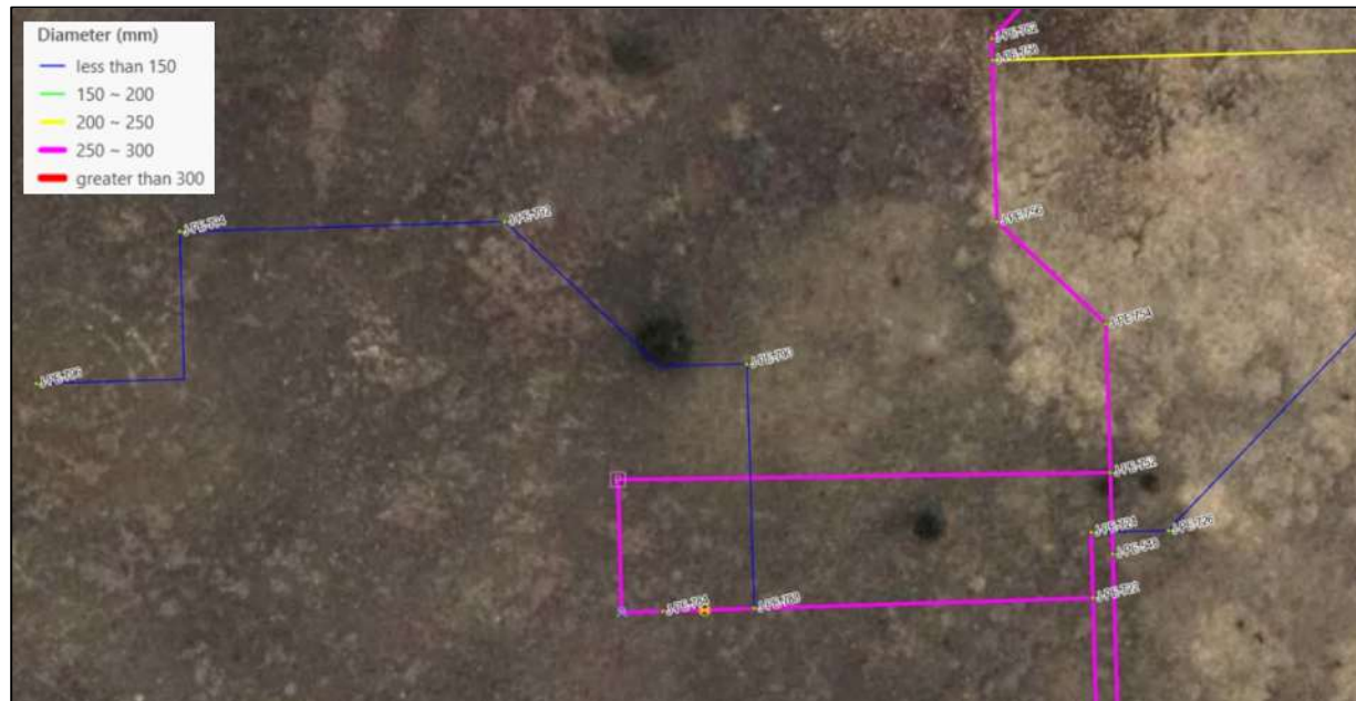
Figure 3-7: Watermain Model Layout Surrounding Fire Pump House
