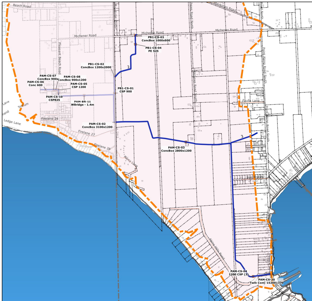
Figure 30 Point Abino Drain Crossings
