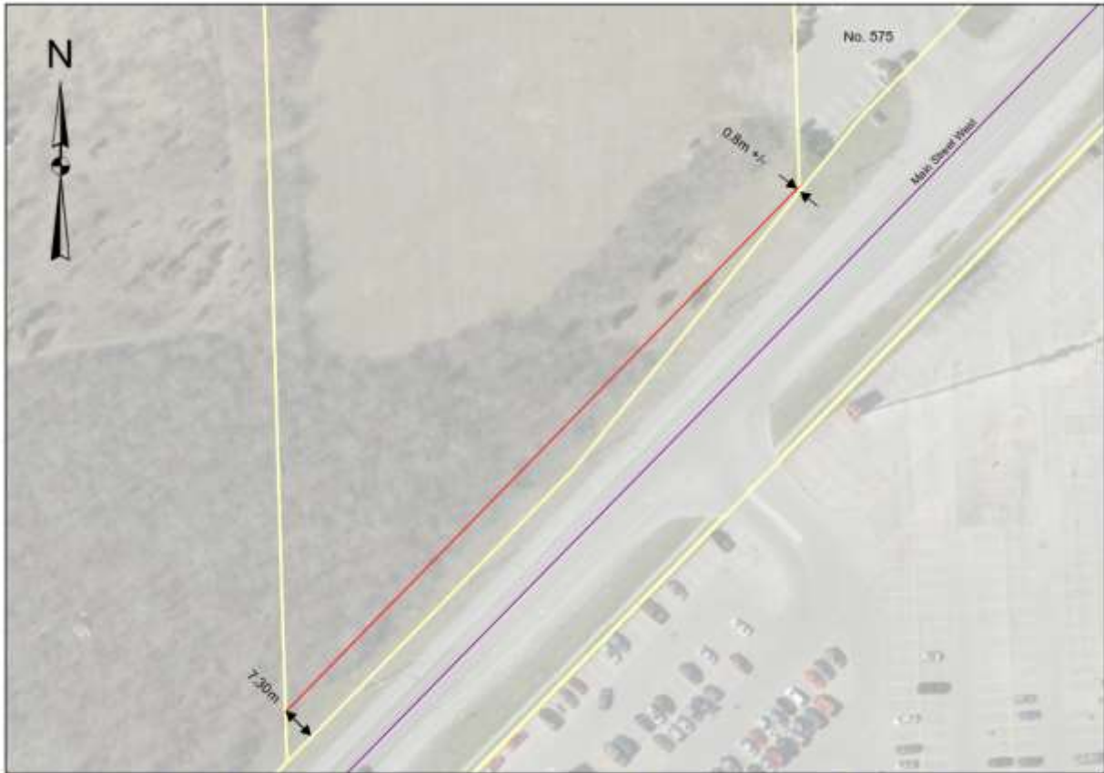
REQUIRED WIDENING TO ACHIEVE A WIDTH OF 17.35 METERS FROM CENTERLINE OF THE ROAD ALLOWANCE FOR MAIN STREET WEST IN PORT COLBORNE
