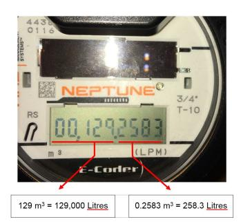
Therefore, 129,258.3 Litres has passed through this water meter since it was installed.
